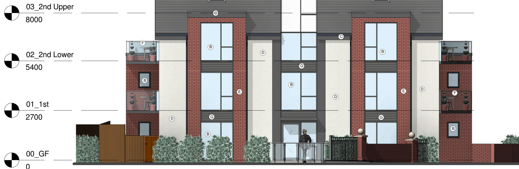
South West Elevation 1 : 100
